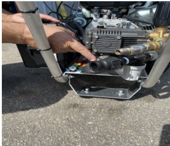
Connect Feed Pump to Water Inlet - Figure #10
