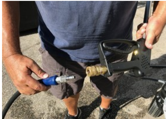
Connecting the gun to the High Pressure Hose - Figure #15
