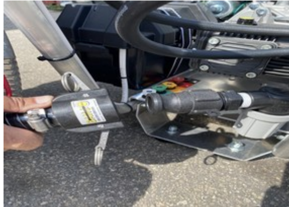
Connect Feed Pump to Water Inlet - Figure #9
